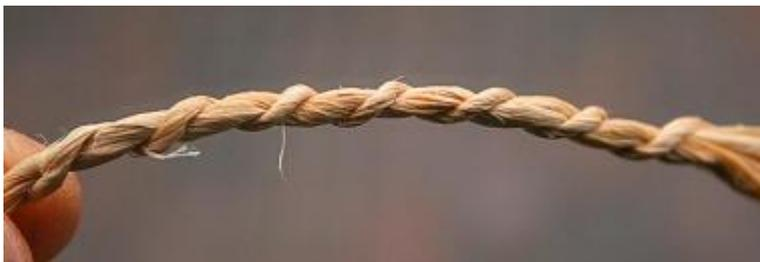
**Example of good cordage** - Each strand is of an equal thickness resulting in a strong balanced cord.
